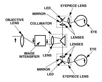
Figure 1-5. Optical Function Diagram.
